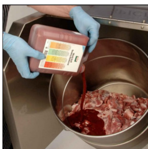
Tumbler (to accelerate the extraction of the muscle proteins)
